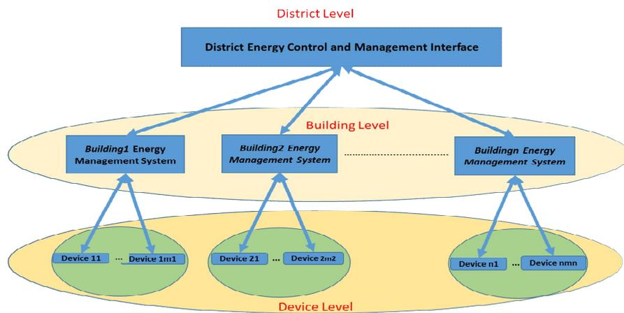
**Fig. 1.** The hierarchical energy management levels in the smart grid.
